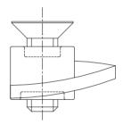
This block is a true representation of a BeamClamp Floorfix. It is designed to allow chequer/durbar plate flooring to be fixed to the supporting steelwork from the top side only with no access to the underside required. As standard it will fix to steelwork up to 15mm thick but can be used with packers to suit any thickness of steel. Please refer to our catalogue or web site for further details of how it works.
